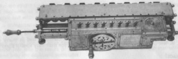
This machine designed by Gottfried Leibnitz was designed to perform multiplication by rapidly repeated additions.
