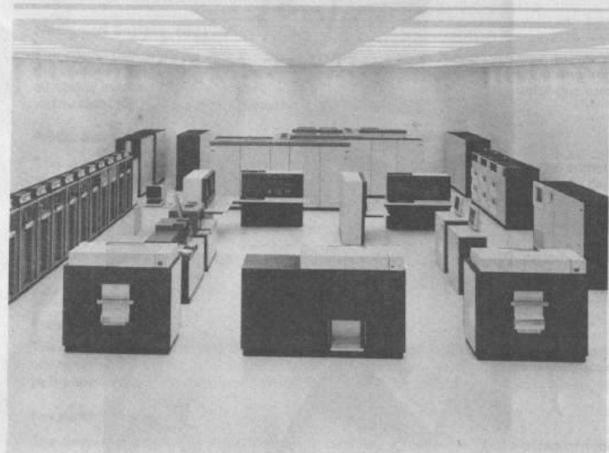
This design model of a modern computer shows magnetic memory disks on the left, output printers in front, and several output display screens that look like television sets.
